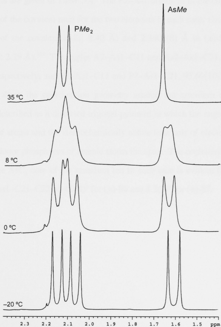
Figure 5.3 Variable temperature 1 H NMR spectra of ( \pm )- 87 in dichloromethane- d 2 .
